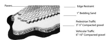
(If more than 6" of gravel is required, then compact in two equal layers)
